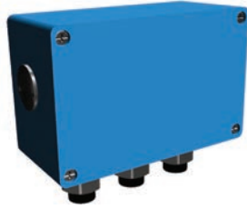
Small auxiliary aluminum terminal box for motor sizes 280-450 (variant codes 418, 568, 380, 569). The size of terminal box ordered with these codes depends on the number of accessories ordered. 80 x 125 mm, max 12 strips. Earthing size M4
